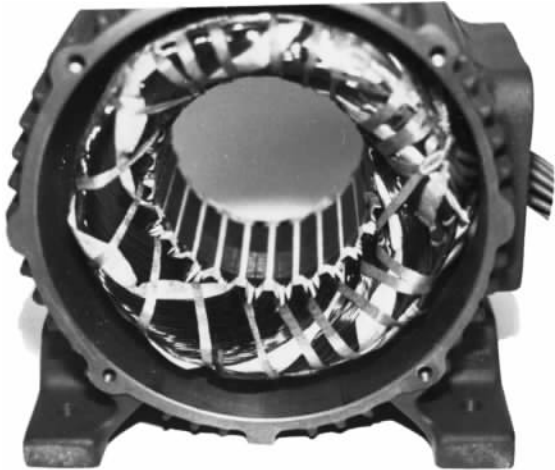
FIGURE 5-1 The stator of a typical induction motor, showing the stator windings. (Courtesy of MagneTek, Inc.)
