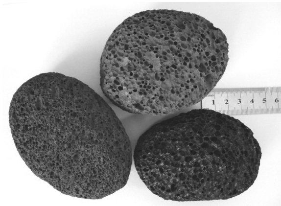
Figure 1.7 An image showing the porous morphology of pumice.
