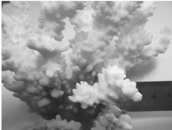
Figure 1.6 An optical photograph showing the porous morphology of coral.
