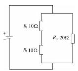
First, use the formula to determine total resistance of the series circuit to find the total resistance of  $R_1$  and  $R_2$ . The following formula is used:
