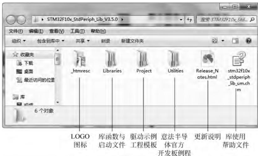
图 3-4 STM32 固件库目录结构
