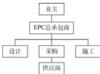
图 2-26 EPC(self-perform construction)合同结构
